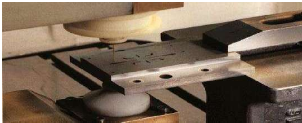
Figure: Wire erosion of an extrusion die
