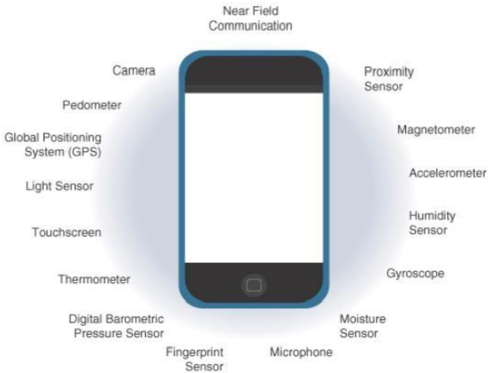
Figure 3-2 Sensors in a Smart Phone
