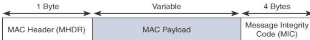
Figure 4-16 High-Level LoRaWAN MAC Frame Format
